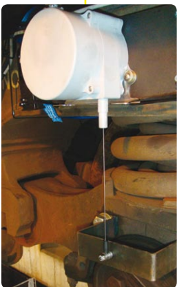
String pot (i.e. on the primary axle, to measure ride quality/suspension system)
