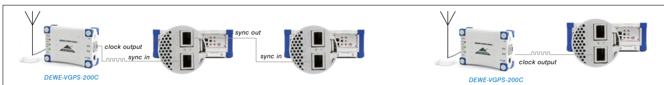
Synchronization of multiple DEWETRON instruments over long distances
