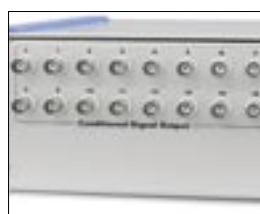
16 BNCs on the rear for conditioned signal output
